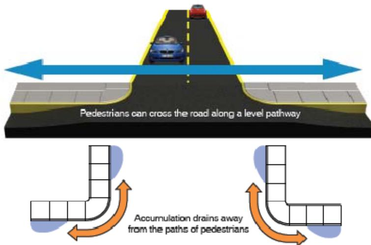
Figure 1: Alternative designs to curb ramps. (a) Current design; (b) Barrier-free pedestrian crossing.
